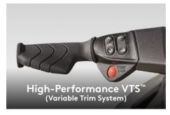
Provides handlebar-activated quick settings so riders can easily find the ideal trim for varying conditions.
