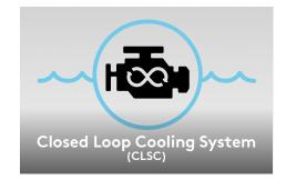
Uses coolant to keep the engine at the ideal temperature, much like a car's radiator. Also keeps out corrosive saltwater and debris.
